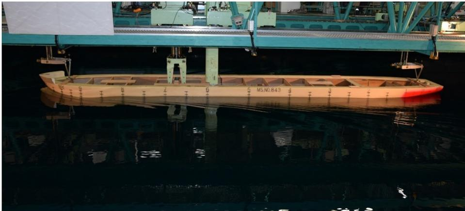
Figure 1: JBC Resistance Test in NMRI Towing Tank.
